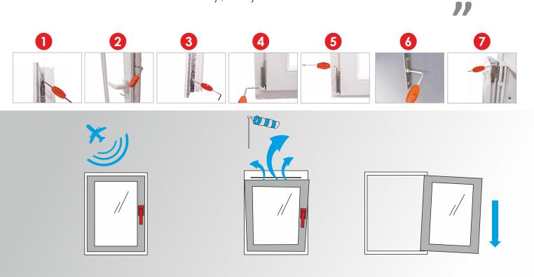
Windows and doors can bend out of shape over time, resulting in loss of gasket pressure and leading to noise and air entering your home. You can easily fix this with an allen key!
